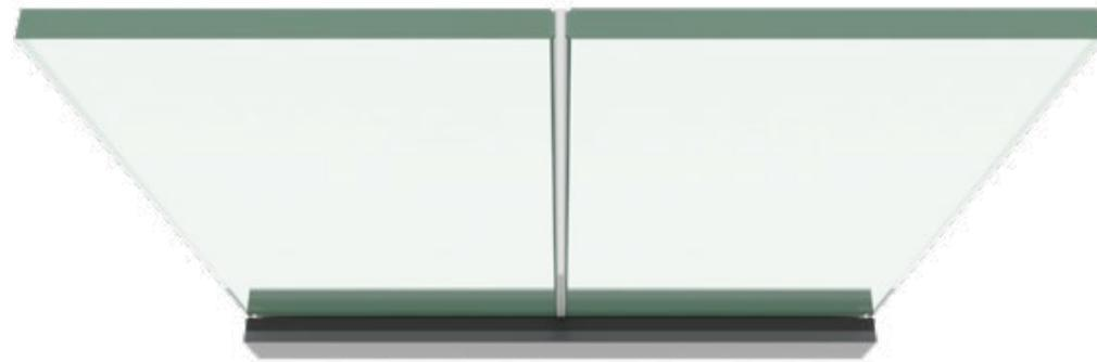
Alignment between the glass modules by means of transparent tape or plastic profiles
